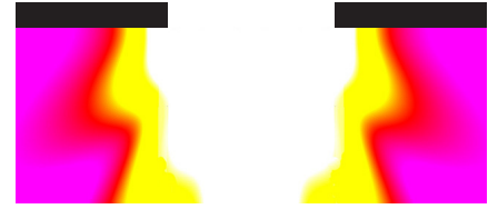
Cross-section of the modelled i-line (365 nm) exposure intensity distribution in a 1 µm thick resist film and a 1 µm slit in the photomask.
