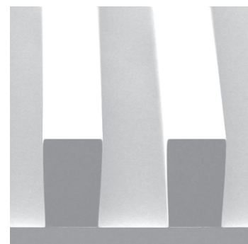
Left: 10 \mu\text{m} lines with a 40 \mu\text{m} thick AZ ® 40 XT; right: 80 \mu\text{m} lines with a 120 \mu\text{m} thick AZ ® 125 nXT. Source: AZ ® 40 XT and AZ ® 125 nXT technical data sheet by AZ-EM.
